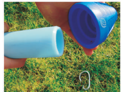
Rura po fazowaniu The same pipe after chamfering
