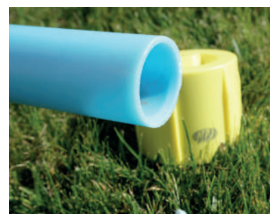
Rura po fazowaniu The same pipe after chamfering
